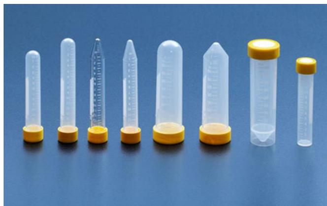
**Fig: Different types of centrifugation tubes**
