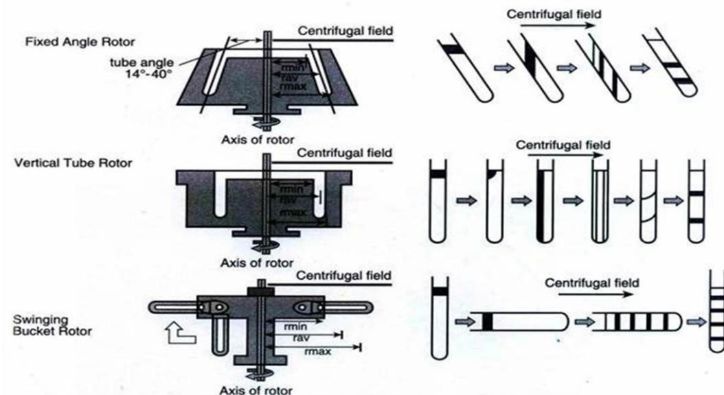
**Fig: Types of centrifugation rotors**
