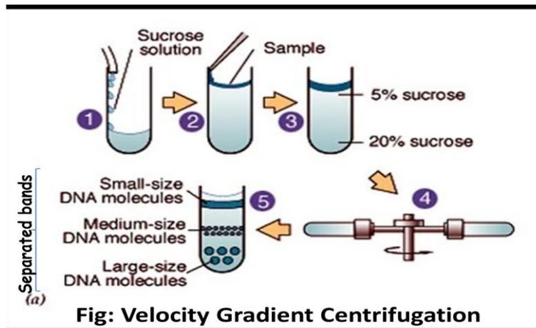
In rate zonal centrifugation, the sample is applied in a thin zone at the top of the centrifuge tube on a density gradient. Under centrifugal force, the particles will begin sedimenting through the gradient in separate zones according to their size shape and density. The run must be terminated before any of the separated particles reach the bottom of the tube.
